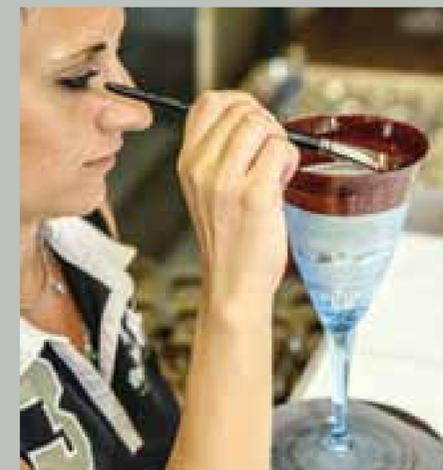
After removing the cover, the band of embossed decoration is painted with a solution of 24-karat gold and fired in a chamber kiln at 560 °C.
