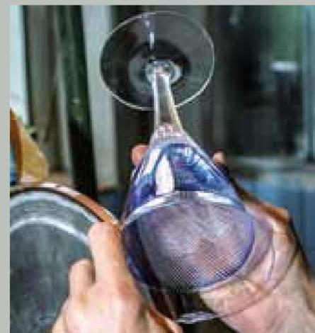
After several hours of cooling in the cooling oven the semi-finished product is ready for cutting. Three types of cut are used on the Splendid set – the stem is cut into edges, a bowl-shaped grinder is used to form a band of bevelled ridges. The most complex is the fine diamond cut, which requires profound concentration, a steady hand and precision work from the cutter.
