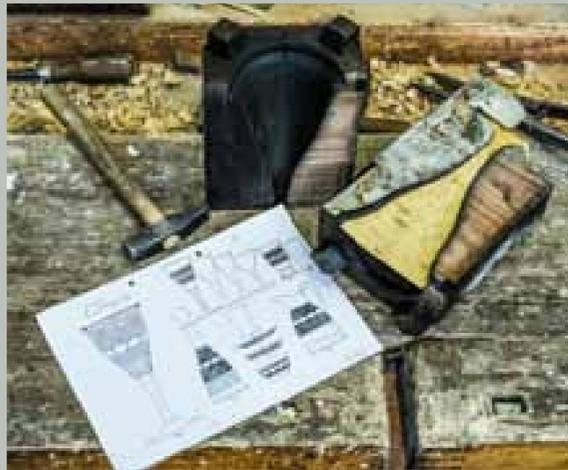
One or more times, depending on the size of the object, the glass master gathers the crystal glass from a pot inside the furnace. The glassblower blows the gathered gob of molten glass into the preformed mould. This can last for several hundred uses.
