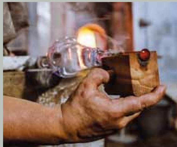
The glassblower forms the glass's stem and base using a special wooden tool.
