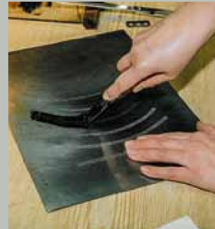
The traditional procedure, patented in 1919, was based on using hydrofluoric acid; it has now been replaced by the more environmentally-friendly technology of sandblasting through the template.
